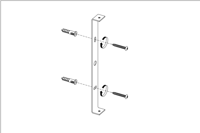
1. Fix the crossbar to the wall by using wall mounting plugs and screws suitable to your wall type.
