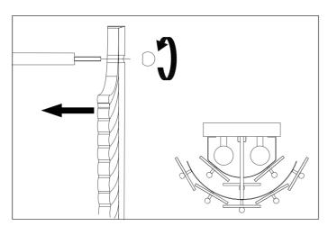
5. Place the glass pcs according to the drawing and secure them with the balls.
