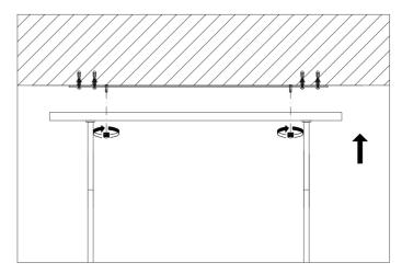
$\boldsymbol{4.}$  Place the ceiling canopy over the ceiling plate and fix it securely with the nuts.
