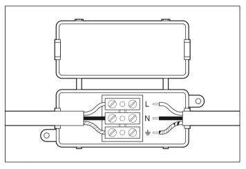
3. Connect the 3 wires according to their colours. Brown is the live wire, blue is the neutral wire, green/yellow is the earth wire.
