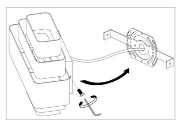
**3.** Place the lamp over the wall plate and fix it securely with the screws supplied.
